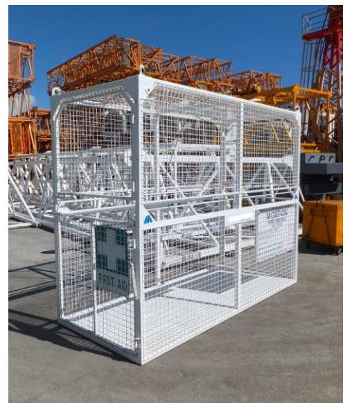
Figure 28 – Compliant first aid box
