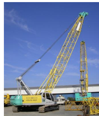
Figure 11 – Lattice boom crawler crane
