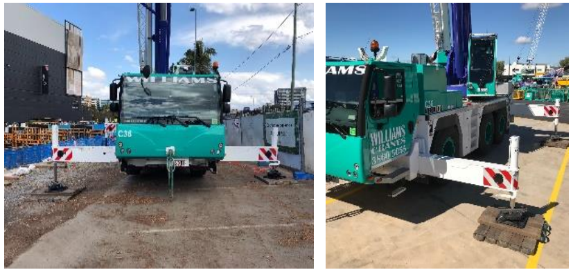
Figure 2 – Hazard striping on a mobile crane
