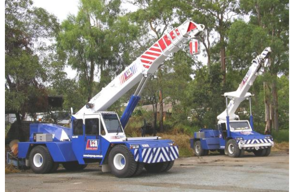
Figure 10 – Pick-and-carry mobile cranes (non-slewing hydraulic cranes)
