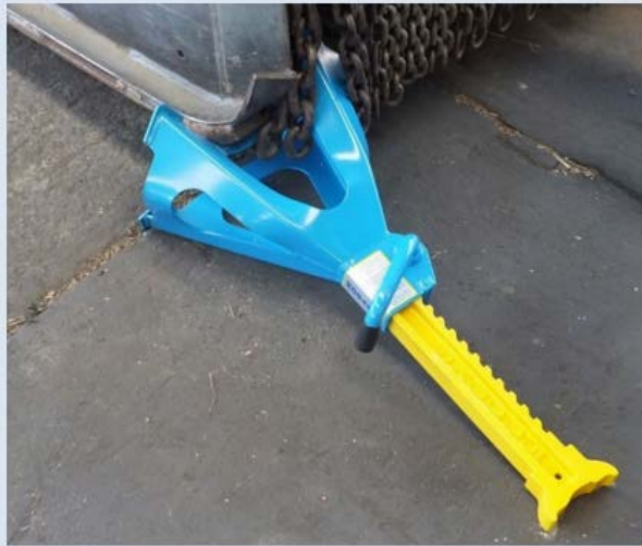
Image 3: Prop base crushed due to force of slasher dropping
