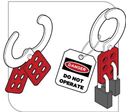
Figure 7: Example of lock-out with a tag and the padlocks of two workers
