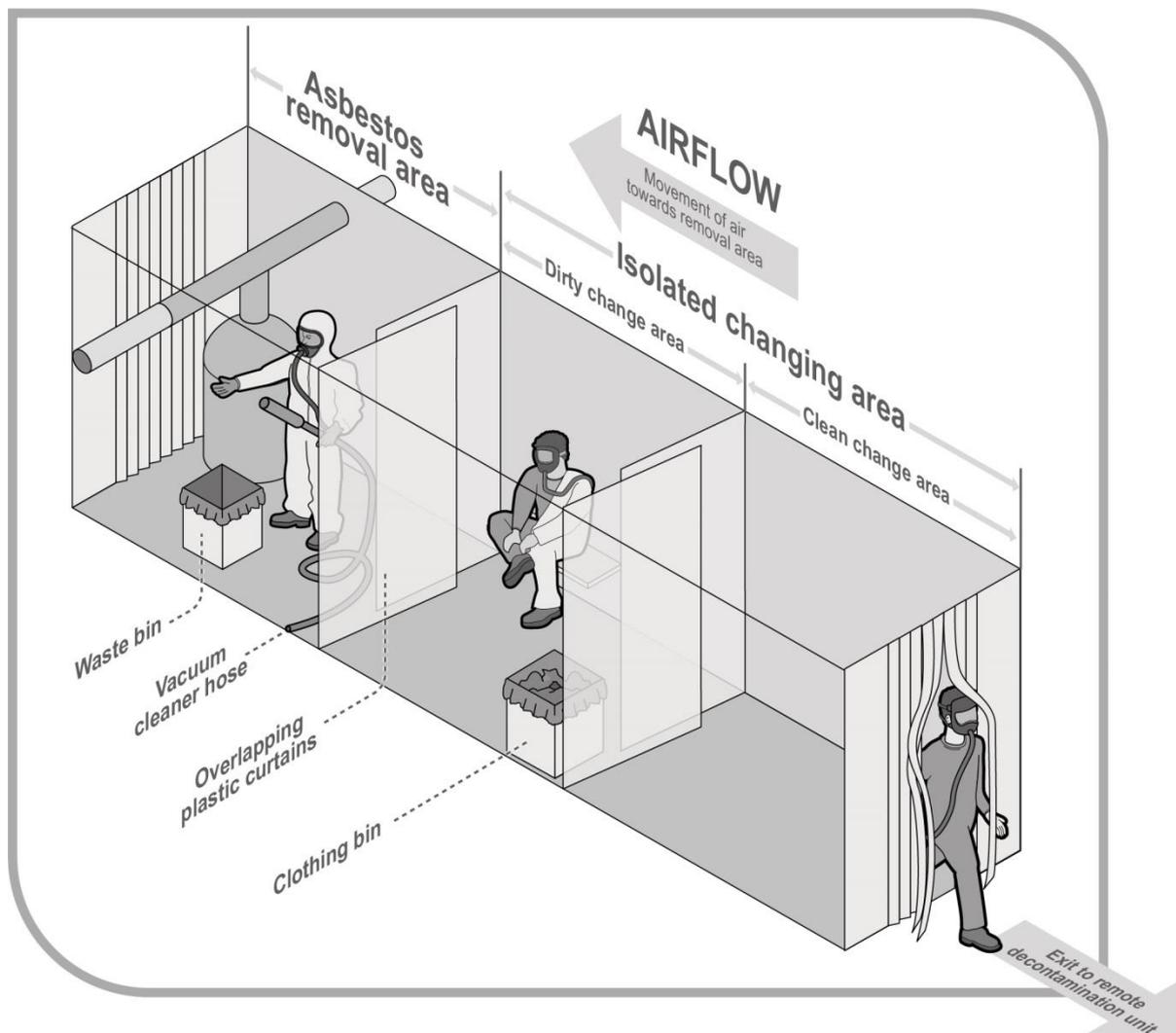
**Figure 5** Preliminary decontamination procedure where a remote decontamination unit is used
