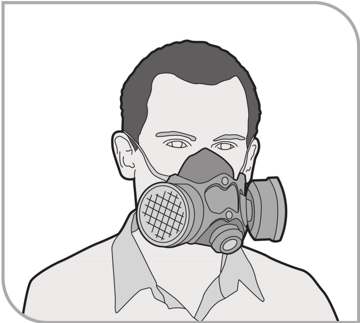
**Figure 10** Half-face particulate filter (cartridge) respirator
